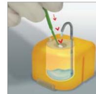
A gentle pressure on the membrane releases the required liquid drop by drop
