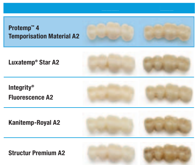
Fig. 9: Coffee test: 3 days immersed in coffee at 36° C.
